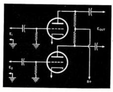
Fig. 2. Circuit for performing subtraction. A necessary requirement is that the two separate inputs be in phase. Circuits of Fig. 1 could similarly be used by employing a 180° phase shift between E, and E<sub>2</sub>.
