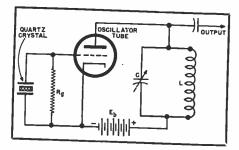
Fig. 9. A fixed-frequency quartzcrystal-controlled oscillator.
