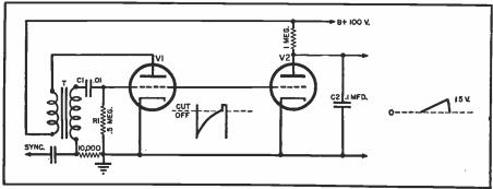
A voltage sweep is usually derived from the slow charge of a condenser through a large resistance and the rapid discharge of the same condenser through a small resistance. Consider the mechanical switching circuit of Fig. 3A. Closing switch 1 will start (Continued on page 106)
