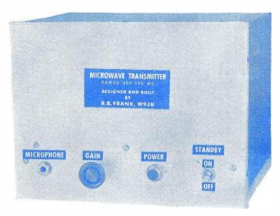
Fig. 1. Although operating at a fixed frequency, this unit may be adjusted to operate at any frequency between 400-500 mc.
