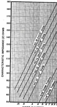
INSIDE DIAMETER OF OUTER CONDUCTOR (INCHES)
