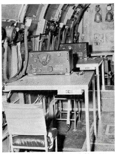
Interior view of the training ship, looking forward towards pilot's compartment. Receiver units of high-powered liaison sets are shown together with sending keys.
