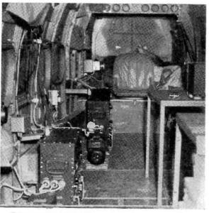
Transmitter units of liaison sets are shown mounted on the floor, where they are easily accessible for tuning.
