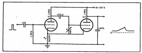
Fig. 12. Wiring diagram of a vacuum-tube single-sweep circuit.
