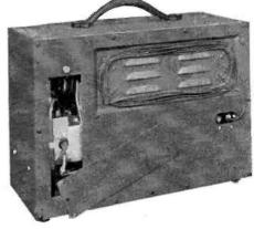
Rear view shows position of coiled antenna wire and a.c.-d.c. line cord.
