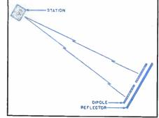
Fig. 7. Illustrating position of dipole and reflector in relation to transmission.
