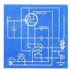
Fig. 5. Diagram of a phototimer.
