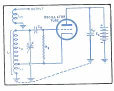
Fig. 3. Modified Hartley oscillator that enables the rotor of the tuning capacitor to be grounded.
