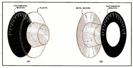
Fig. 2. Two methods of obtaining a professional-appearing calibration. (A) The photographic negative with the calibration marking appearing thereon is glued to the panel or to the back of the flange. A transparent plastic knob is used with this arrangement. (B) Photographic negative is glued directly to the knob flange.
