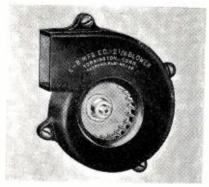
bottom. Operating under all conditions of climate and temperature, the unit which weighs but 3½ ounces, delivers 50 cubic feet per minute at 8000 r.p.m. It is available with shaft bores of either .1895 or ¼",
