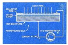
Fig. 6. Circuit of an exposure meter.
